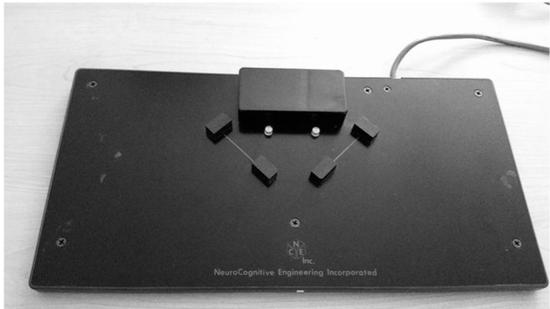
Fig. 1. Light beam finger tapper (NeuroCognitive Engineering). The apparatus consists of two light beams, one on each side of the board, which project about 1 mm above the board between two raised nodules. Gray lines between the right-side and left-side modules cue respondents where to place their index finger during a test trial. Lowering an index finger through the beam registers the tap. A computer-based software program administers the task and captures the number of finger taps and inter-tap intervals during a 10-s trial of finger tapping
